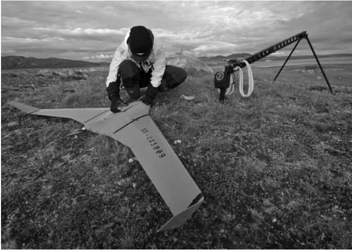
Nejc prepares the C-ASTRAL BRAMOR UAV for an orthophoto flight over Ikpik
